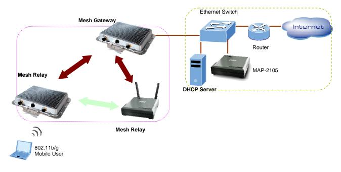
The MAP-2105 should connect to the network that provide DHCP services (the first time installation) In this guide, we will base on XRT-401D (Internet Broadband Router) as the example for DHCP server, switch and router, this installation can vary on the network planning.
